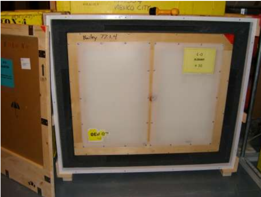
(fig. 4-5) WMAA Standard (upright) crate (pre-Whitney Green) with Travel Frame. Note the Corrugate on the outside of the travel frame and registration mark on the lid.
