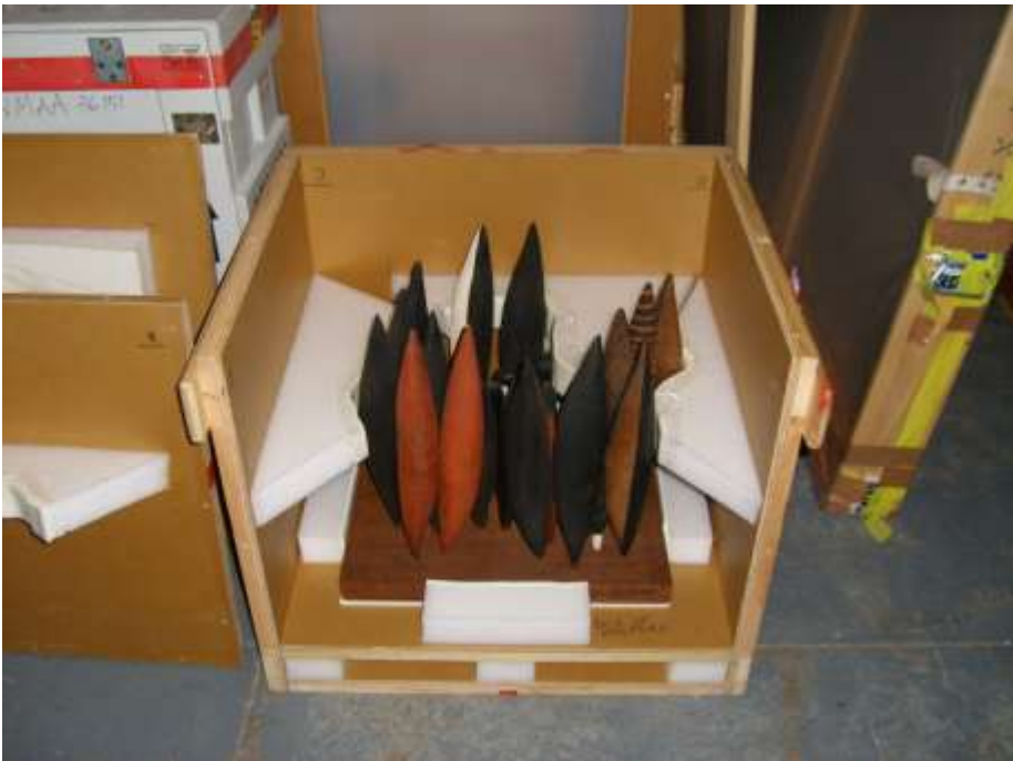
(fig. 19) Note Ethafoam is covered in Volara and then Dartek at contact points.
