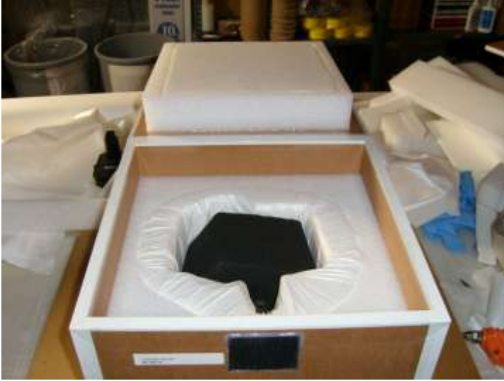
(fig.14) Example of a cavity pack in an inner box. The element is packed in Ethafaom and Nomex.
