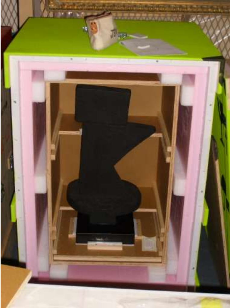
(fig.7) WMAA standard crate with inner crate to house sculpture. Note: Artwork is placed on a well designed sliding tray.
