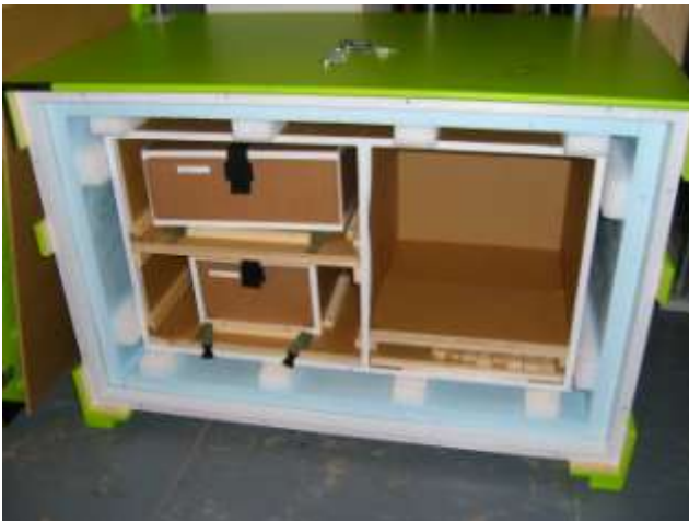
(fig. 8 ) Standard crate with inner crate to house boxes and sculpture. Note: This crate is made to house one complete sculpture, the boxes are constructed using archival materials inside.
