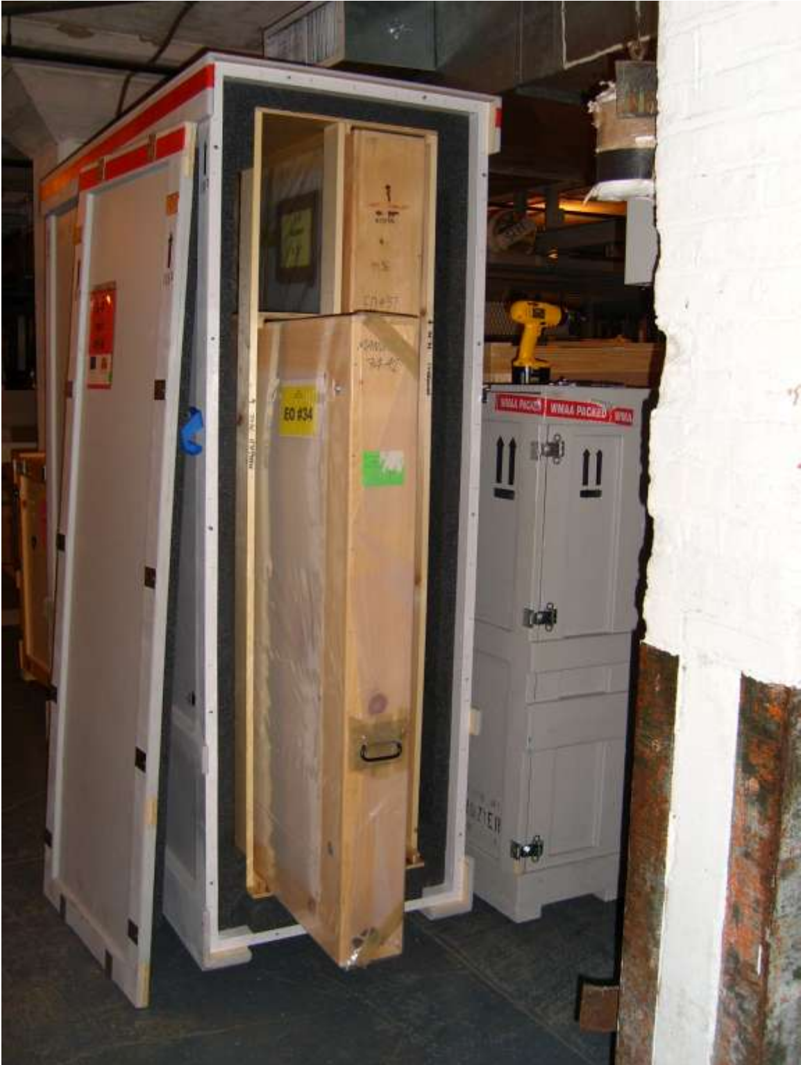
(fig. 3) Example of WMAA End Load Crate loaded with Travel Frames. Note cage structure of interior.
