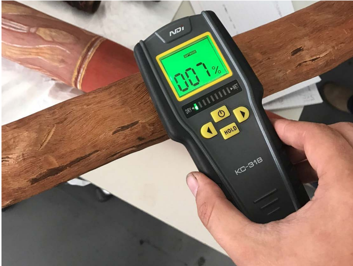
Figure 8.2 Monitoring moisture levels in the instrument. © South Australian Museum. Author: Alice Beale.
